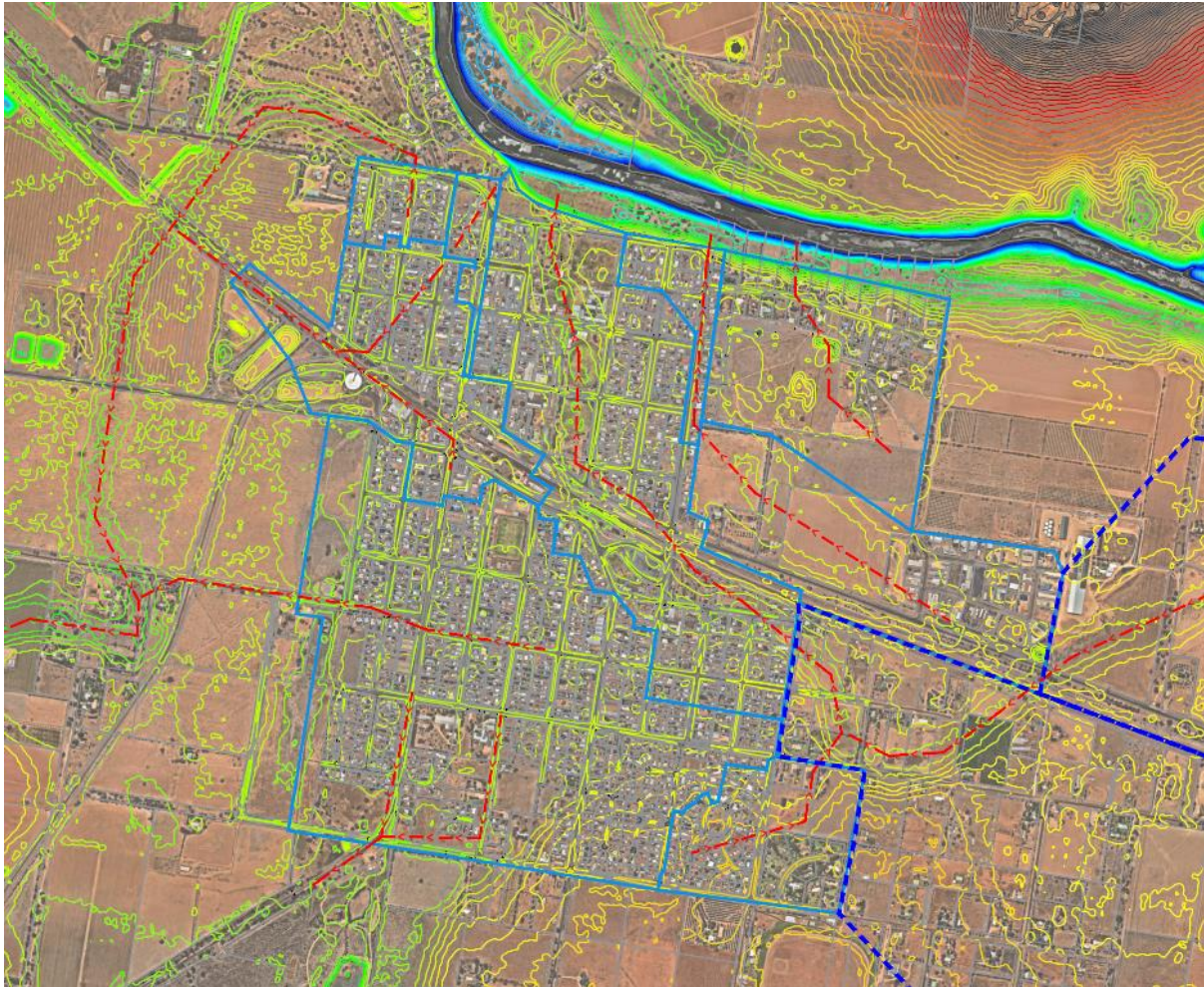
Figure 2 Existing Topography showing existing catchments (blue) and landform overland flowpath (red)
